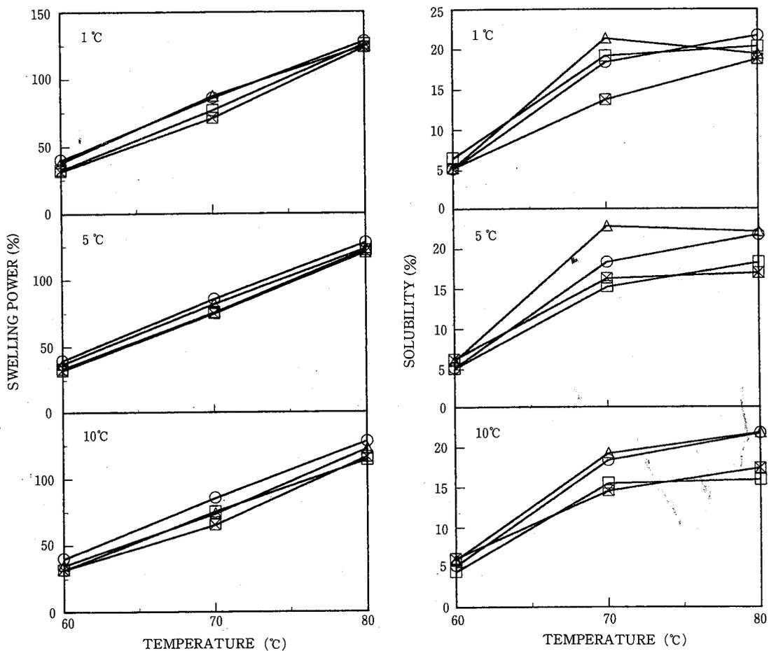
Fig. 1. Swelling power and solubility patterns of potato starches from tubers stored at different temperatures for 1 ( $\Delta$ ), 4 ( $\boxtimes$ ), 6 ( $\square$ ) months; ( $\circ$ ) control. Values are means of two replicates.
