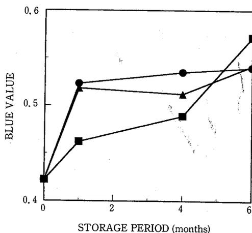
Fig. 3. Blue value of potato starches from tubers stored for 6 months at 1°C (■), 5°C (●), and 10°C (▲). Values are means of two replicates.
