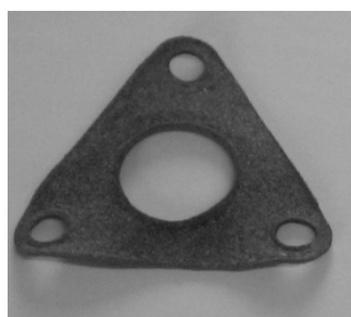
Figure4. Deformation of cork gasket material
