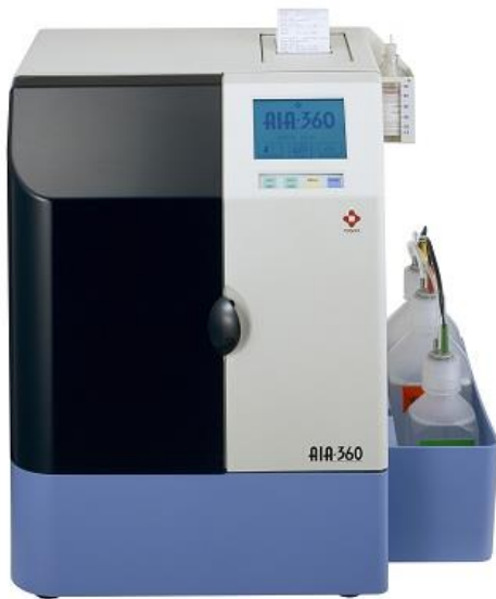
Fig2-5 Automatic EIA device to measure equine blood hormone concentrations in this study.
