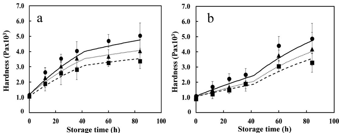
**Fig. 3.** Comparison of simulation curves and experimental data on hardness of breads stored for 84 h in the step-up and step-down change conditions of bread storage temperature.<sup>1)</sup>
