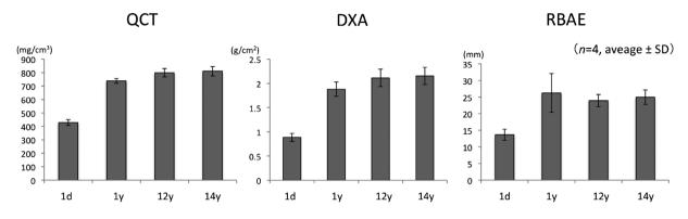
Fig. 5. BMD values at different ages (14, 12 and 1 year of age and 1 day of age) as measured by QCT, DXA, and RBAE. QCT and DXA measurements exhibited a similar pattern, but RBAE could not distinguish between 14-, 12- and 1-year-old bone.
