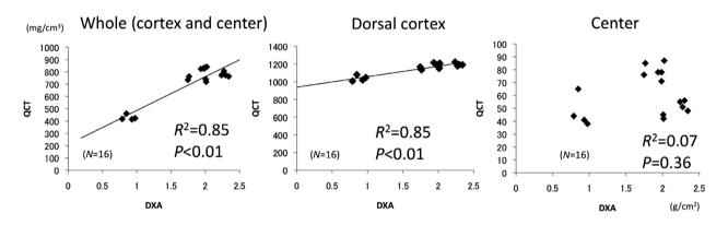
Fig. 3. Comparison of BMD values as measured by QCT and dual energy X-ray absorptiometry (DXA). There were strong correlations for the whole bone (cortex and center) and dorsal cortex, but not for the center.
