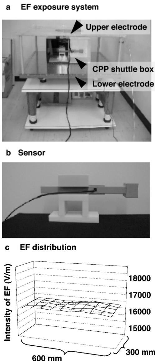
Fig. 1. Electric field (EF) exposure system (a). The shuttle box consisted of white and black color compartment were placed on the center of lower electrode of EF exposure system. Distribution in intensity of electric field (EF) on the bottom of shuttle box placed on center (c).
