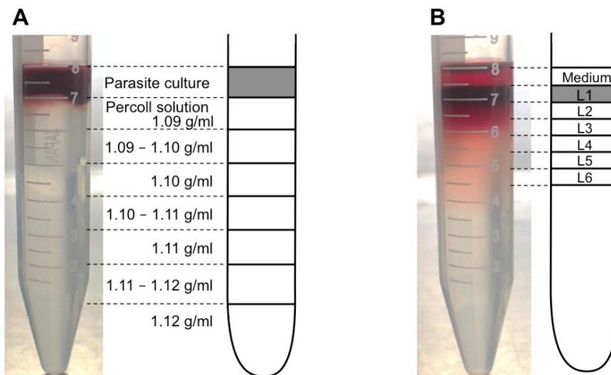
**Fig. 1.** Percoll density gradient. (A) Parasite culture and Percoll solution having densities from 1.09 to 1.12 g/ml before centrifugation. (B) After centrifugation, resulting in six different layers.
