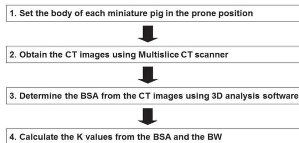
Fig. 1. The measuring method using a CT scanner.
